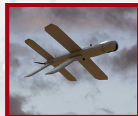
The Lancet-3 is a Russian loitering munition with two sets of X-shaped wings and an electric propeller propulsion system. Image from Shutterstock.
